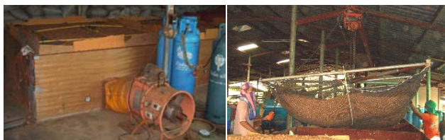
Taiwan-type dryer used for bulk drying of unpeeled longan, loaded with three layers of longan fruit, each 20 cm high.
