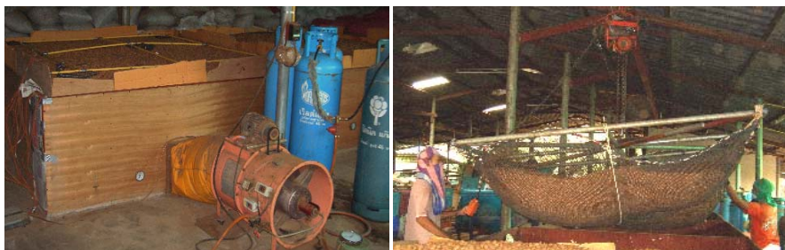
Figure 1. The Taiwan-type dryer for bulk drying of unpeeled longan, loaded with three layers of fruit each 20 cm high.
