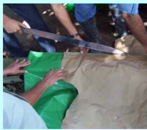
Manual adaptation: Plastic tube is cut to appropriate size and sealed using a hot machete
