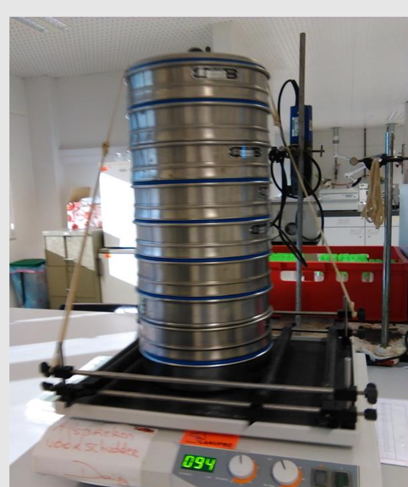
Fig 1. Sieving of wheat bran with shaker for determination of particle size distribution
