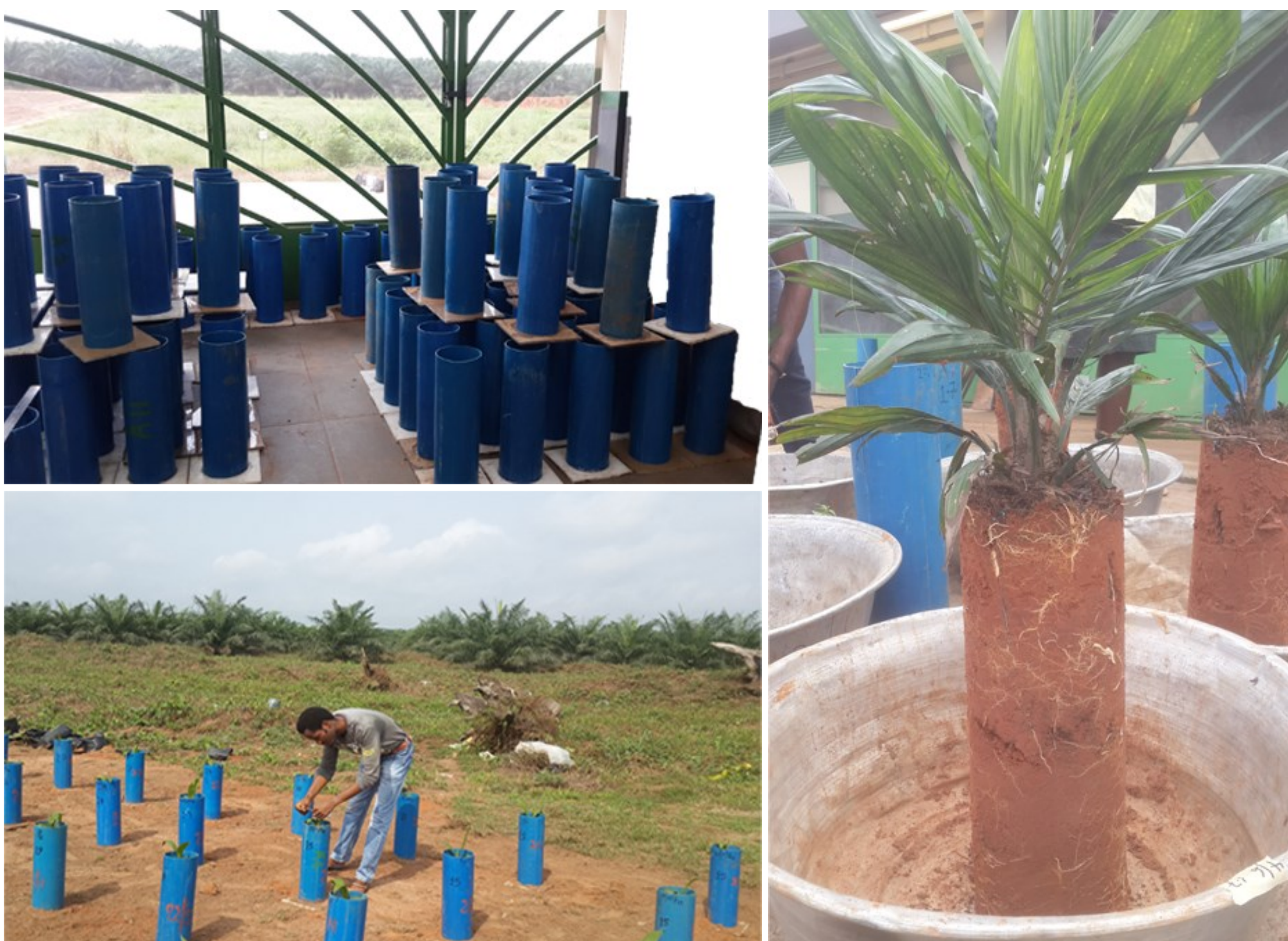
Figure 2 : Packed pipes prior to soil filling and compaction (top left), Growth observation of seedlings during the early trial stage (bottom left) and exposed soil cylinder with roots ready for biomass data collection (right)
