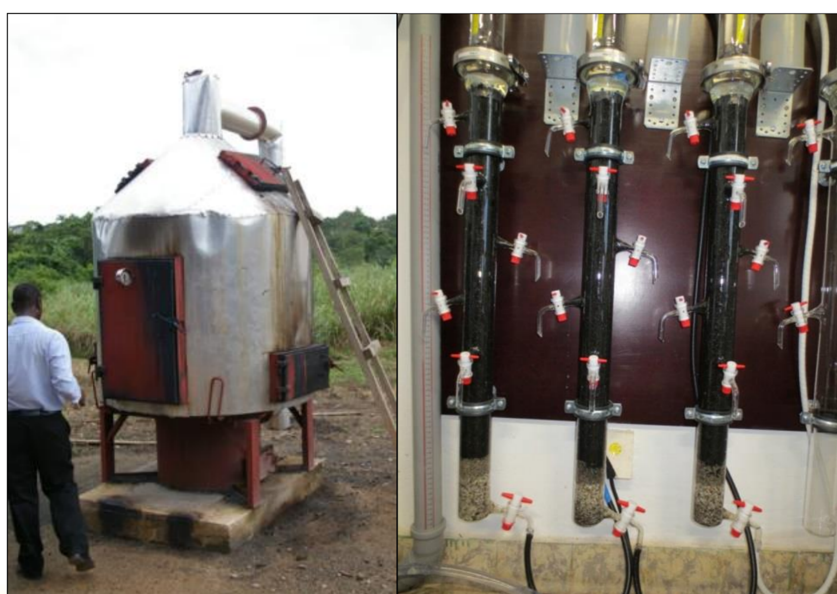
Fig. 5: Left: Custom biochar kiln. Right: Filtration columns with biochar
